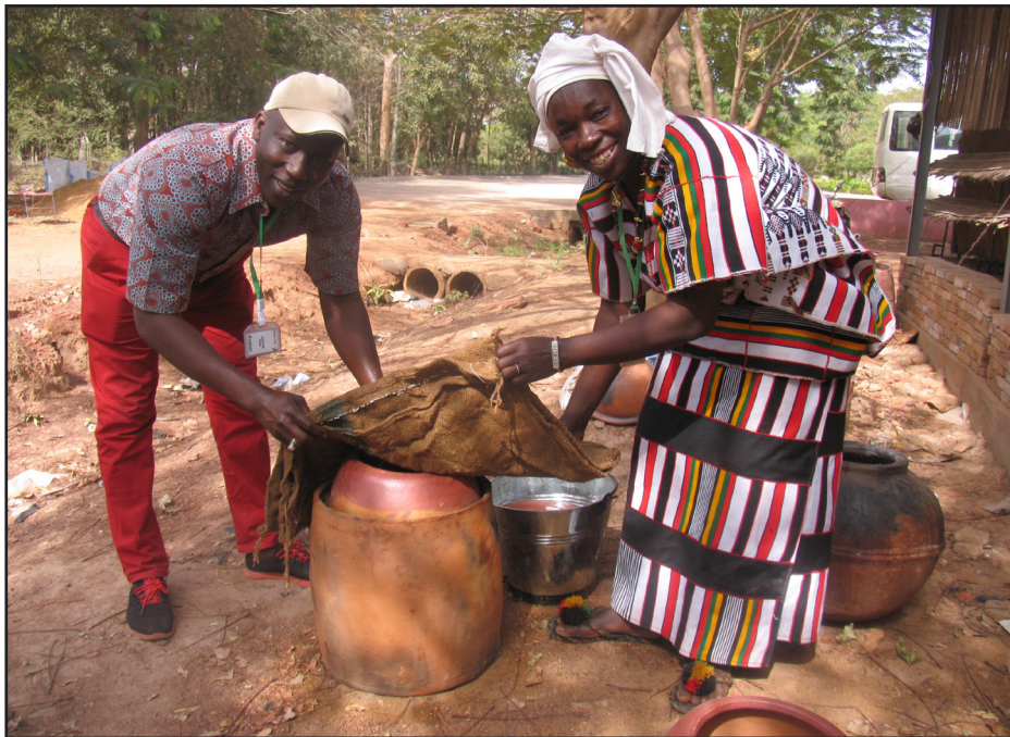
Djiguiba Boureima (Left) and Kadidia Nienta (Right) assembling a clay pot cooler in Samanko, Mali; Photo credit: Ba Germain Diarra
